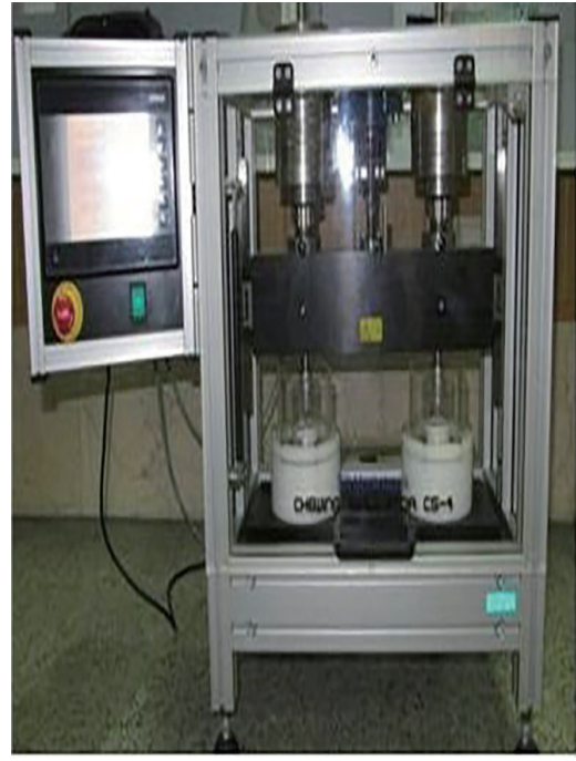
Fig. 3. Cyclic loading was applied to imitate the oral condition.
