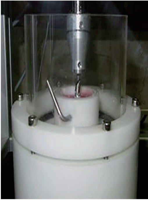
Fig. 2. The forces are applied in 45-degree angle over the crowns.
