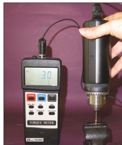
Fig 3 Torque application with electronic torque meter.
