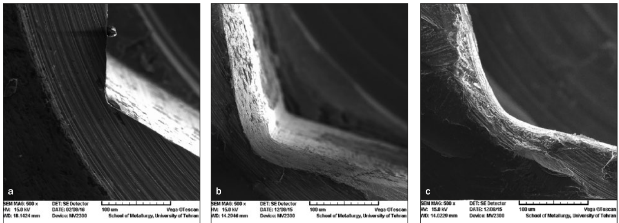
Fig 9 SEM micrographs ( \times 500 magnification) of internal hexagonal slot of screw head before loading for (a) unused screw, (b) after five I/R cycles, and (c) after 15 I/R cycles.
