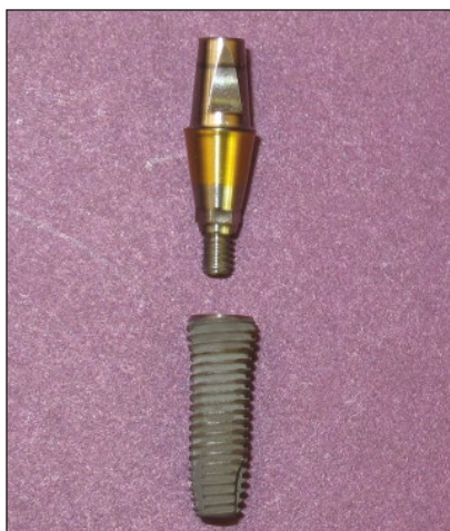
Fig 1 Implant, abutment, and abutment screw used in this study.
