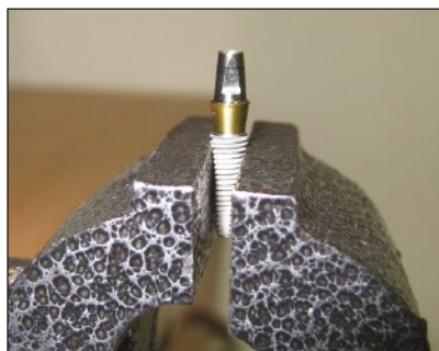
Fig 2 Mounting jig that tightly holds implant.
