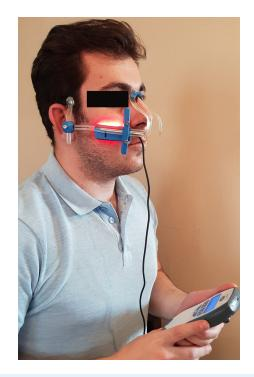
Figure 2. LED OsseoPulse and Patient Using the Device.
