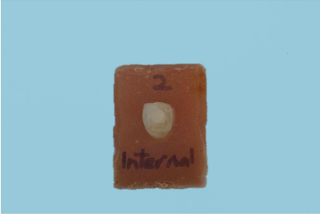
Figure 1. Specimens mounted in blocks of auto-polymerizing acrylic resin
